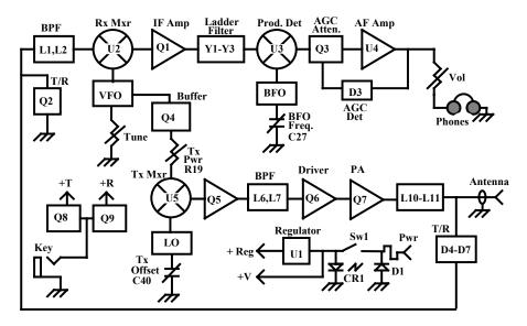
In transmit, buffer Q4 samples U2's VFO signal and feeds it through attenuator R19 to transmit mixer U5. Q5 boosts U5 output, and Chebechev filter L6-L7 selects the desired mixer product. Driver Q6 boost the filtered signal and feeds it through an L network to class-C PA amplifier Q7. +T switch Q8 is keyed to generate CW characters. This powers U5, Q5, and the bias line to Q6. Pi-filter L10-L11 reduces transmitter harmonic content.
