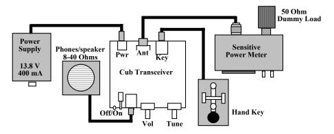
If no RF power meter is available, install a dummy load at the *cub* 's antenna jack and connect a 5mm LED across the antenna terminals (LED polarity not important). This will serve as a relative power indicator.
